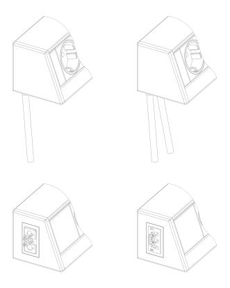
Fixed Power Supply Cable through the bottom of the profile
