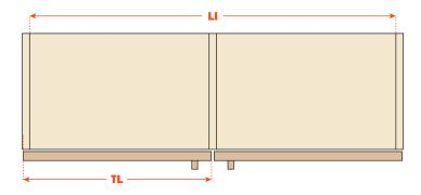
The handle should be placed close to the leading edge of the door, or at a maximum distance of one third of its width (TL).
