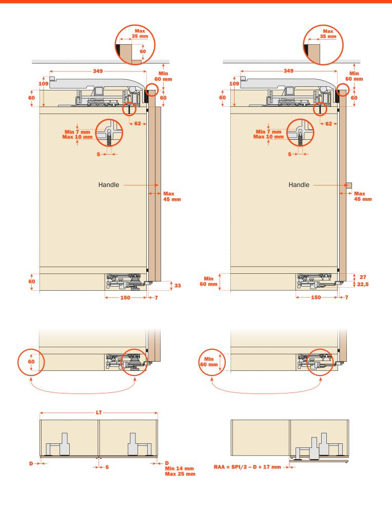
Slider L70 Flex is a flexible system that can be adapted to the internal width of the unit ( $\mathbf{LI}$ ) with a minimum of 1731 mm to a maximum of 3400 mm.
