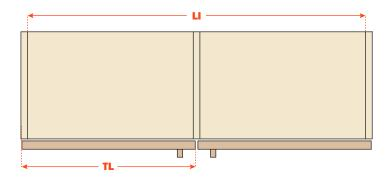
The handle should be placed close to the leading edge of the door, or at a maximum distance of one third of its width (TL).
