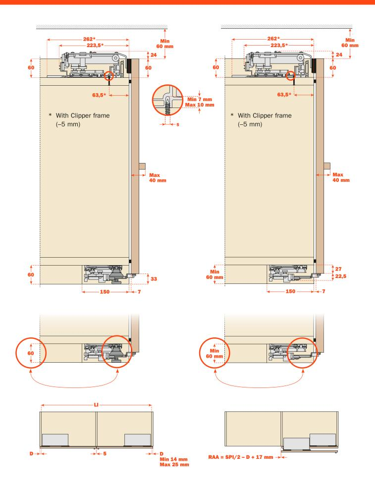
Slider M50 Flex is a flexible system that can be adapted to the internal width of the unit ( $\mathbf{LI}$ ) with a minimum of 1531 mm to a maximum of 3200 mm.
