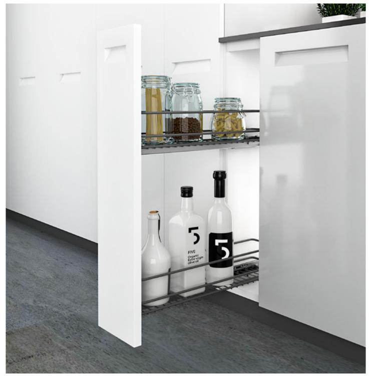
Full extension runners with soft close system (332) Single extension runners with soft close system (332S) Three-dimensional adjustment of the door Total load capacity: 30 kg (332), 25 kg (332S) Possibility to have the runners on the left, on the right side or crossed Bottle holder dividers available on demand Wall-cabinet version available on demand
