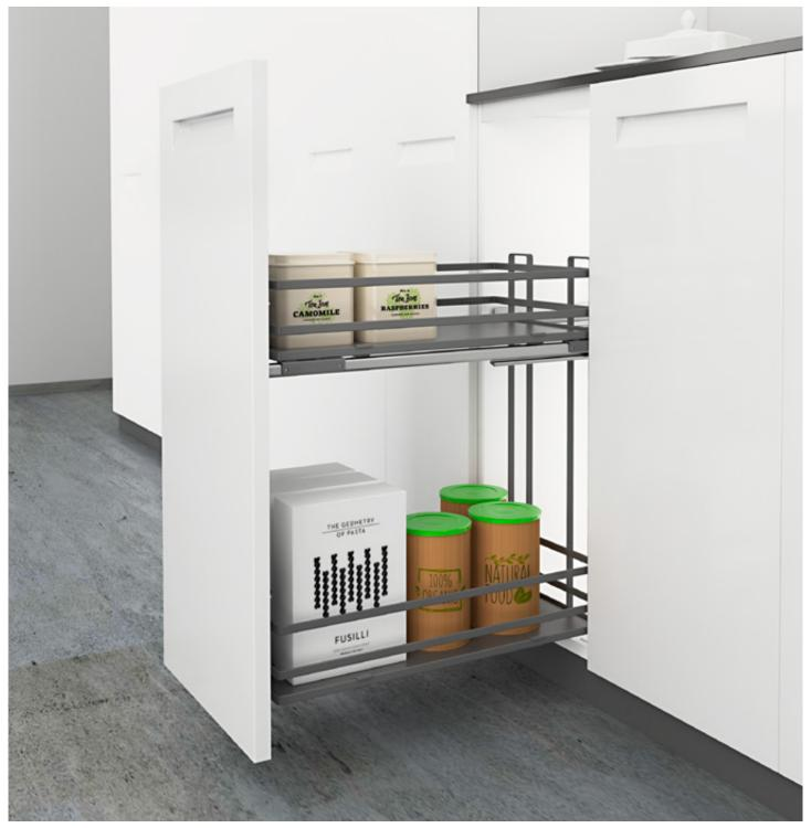
Full extension runners with soft close system Three-dimensional adjustment of the door Total load capacity: 30 kg Fixing position of the runners on the sides of the cabinet Installation depth: 480 mm Installation height: 506 mm
